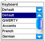
Keyboard allows you to choose the layout of the unit's virtual keyboard. You will use the virtual keyboard when entering information for some of the unit's Find screens. See *Using the Virtual Keyboard* in Section 5. A drop down box will appear when you press the arrow key under the Keyboard header. Use the slider to scroll through the drop down box list and make your selection.
